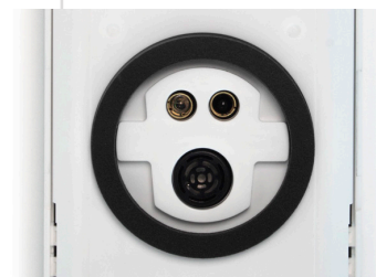
The underside of the GT 1210, with integrated cargo sensor and tamper detection seal.
